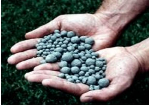
Clinker is discharged red-hot from the lower end of the kiln and generally is brought down to handling temperature in various types of coolers. The heated air from the coolers is returned to the kilns, a process that saves fuel and increases burning efficiency.
