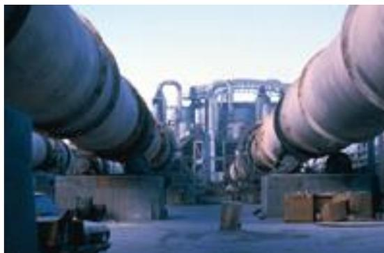
As the material moves through the kiln, certain elements are driven off in the form of gases. The remaining elements unite to form a new substance
